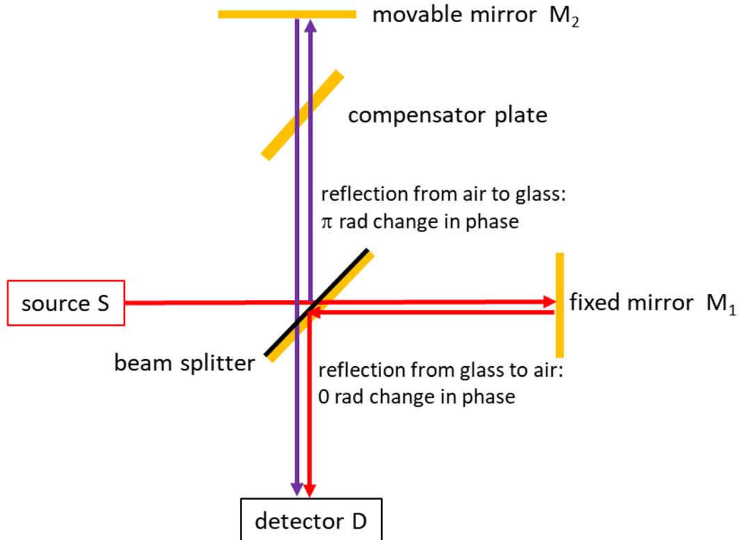
Fig. 1. Michelson interferometer.
