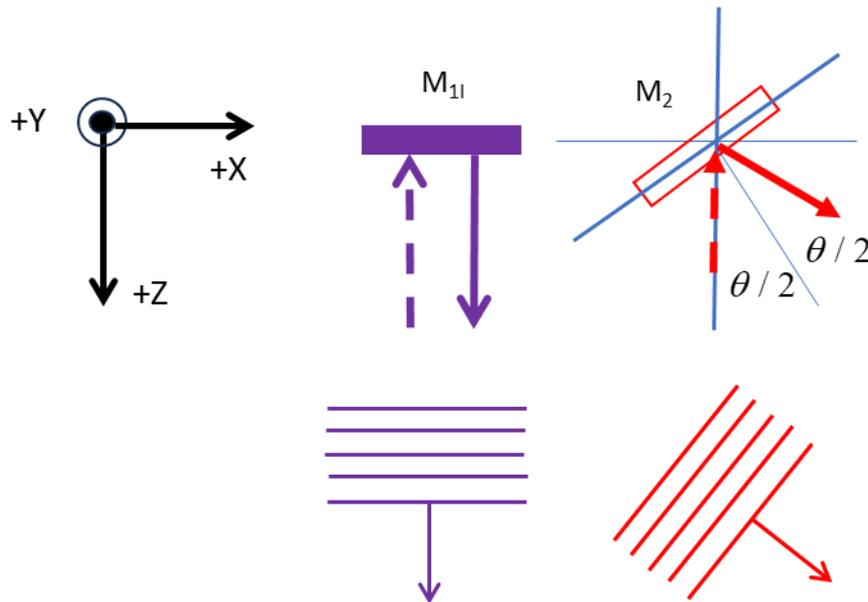
Fig. 3. Mirror geometry for a tilted movable mirror  $M_2$ . The mirror  $M_2$  is tilted through the angle  $\theta/2$  w.r.t. the Z axis, while the beam is deflected through an angle  $\theta$ .
