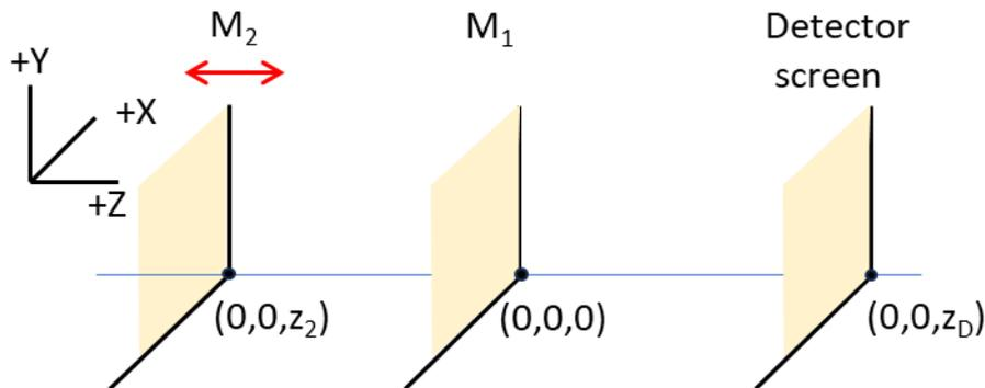
Fig. 4. Geometry of a Michelson interferometer for calculating the detector screen intensity from the electric fields propagated from each mirror.
