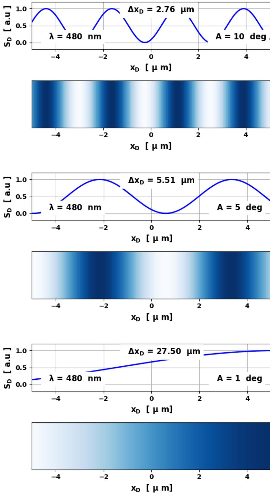
Fig. 6. When the tilt angle decreases, the fringe separation becomes smaller.  $\theta \rightarrow 0 \quad \sin \theta \rightarrow 0 \quad \Delta x_D \rightarrow \infty$  [emMichelsonD.py](#)
