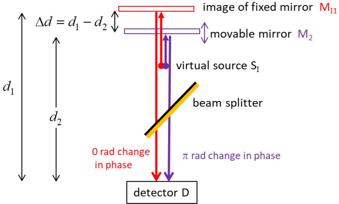
Fig. 2. Linear optical equivalent arrangement of the Michelson interferometer.
