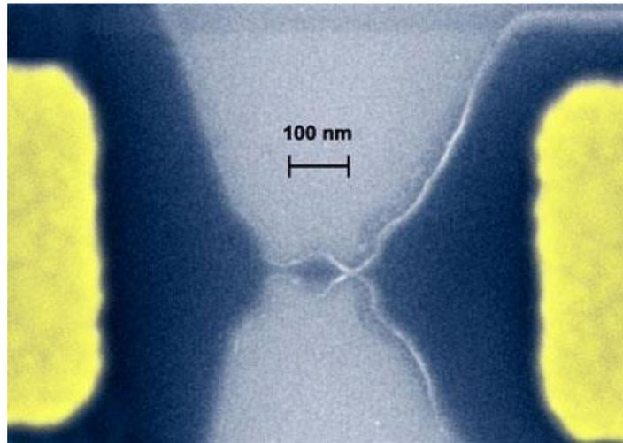
Fig. 1. Quantum dot carved from a graphene sheet
