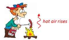
Energy is transferred to the sausage from the fire by natural convection – hot air is less dense than surrounding air and rises
