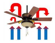
In the summer, ceiling fans rotate anticlockwise to mix warm air and force a cool breeze downwards, creating a downdraft.
