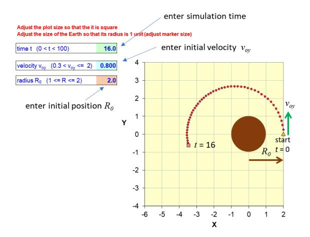
The EXCEL Worksheet is used for a simulation of the motion of a satellite around the Earth. To simplify the calculations, the product  $GM_E$  and the radius of the Earth  $R_E$  are set to one  $(GM_E = 1 \quad R_E = 1)$ . The location of the Earth is at the Origin (0,0) and corresponds to a focus point of the ellipse.
