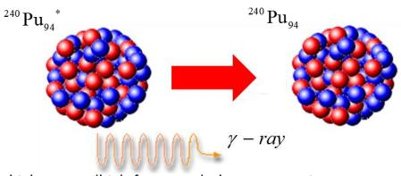
high-energy (high-frequency) electromagnetic wave
